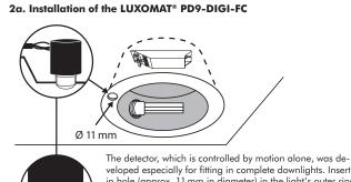
veloped especially for fitting in complete downlights. Insert in hole (approx. 11 mm in diameter) in the light's outer ring. Then connect detector with power supply using RJ11 plug. PLEASE NOTE: The black protective cap must not be removed otherwise malfunctions may occur.
