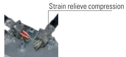
The cable is fixed to the cable clamp by a strain relieve compression. Cable clamps are available in diameter from 6 up to 12 mm. This allows to connect cables of any diameters, 6 up to 12 mm. If necessary, we recommend the use of heat shrinking tube to adjust the cable diameter to the cable clamp. In this case a verification of the strain relieve with a test force of at least 150 N during 1 Minute shall be considered.
